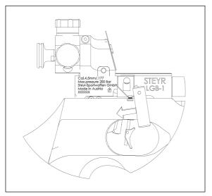
2.) The filled magazine has to be fully inserted from the right to the left in the magazine port. The rifle is now ready for firing.
