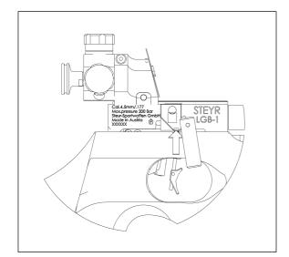
PLEASE NOTE: The magazine may also be removed without emptying it. When pressing the magazine catch, ensure the magazine, which is under spring pressure, dows not fly out.
