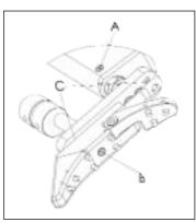
The plate of the butt plate can be adjusted in 2 different heights by loosening screws A. Additionally the plate can be adjusted in two different angles: 90° and 80°.
