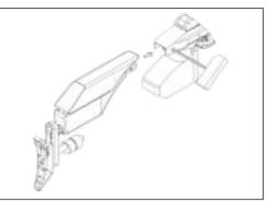
Push the barrel shroud against the spring pressure on the barrel and twist it into place against the bayonet lock.
