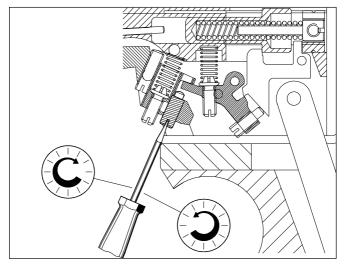
To reduce first stage travel, first loosen the triggerstop screw counterclockwise a few turns.
