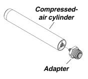
Open valve of refill cylinder to charge the compressed-air cylinder with compressed-air (make sure to use only dehumidified compressed-air).
