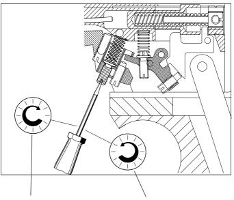
Turning the screw clockwise increases the first stage pressure
