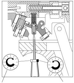
Turning screw clockwise increases the second stage pressure;
